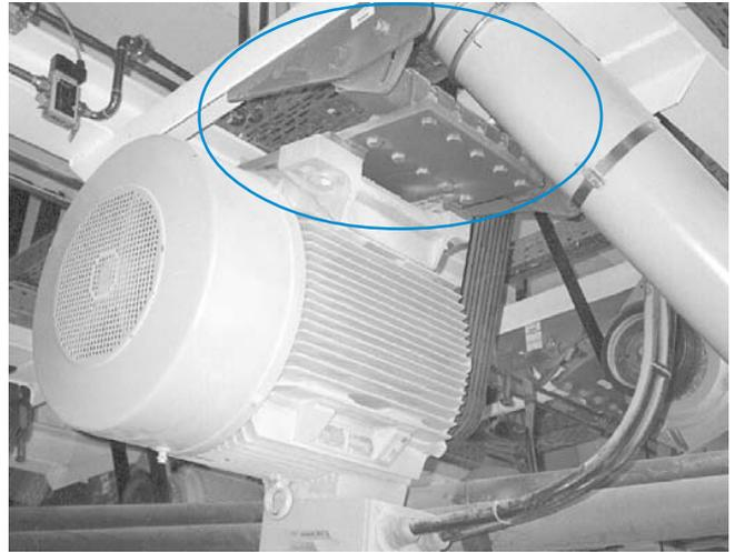
50HP motor to flour-mill on MB 50 (hanging installation)
