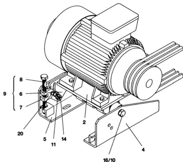
4. Turn jacking bolt M 20 (8) counter-clockwise to tension the belt(s). Check the belt tension with the data specified by the belt manufacturer or according to the test force table on page 83.
